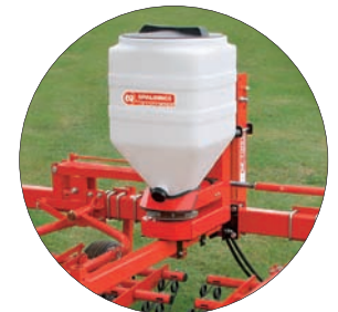
The Tined Weeder can be fitted with the Spaldings Broadcaster to give maximum spreading flexibility for grassland and arable applications.
