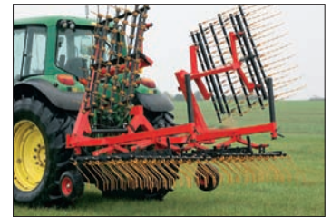
Twin hydraulic rams for quick folding with bushed pivots on folding wings for long life.
