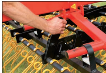
Quick and simple tine rake adjustment via a five positional lever. Easy tine angle adjustment for use in all ground conditions.
