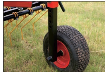
Two fully adjustable pneumatic depth wheels (with the option of 4) for maximum effectiveness.
