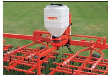
Ideal for re-seeding grassland when mounted on Spaldings 6m Tined Weeder.
